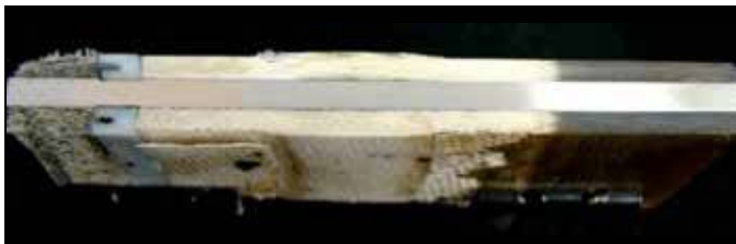
Steam attack on GRE isolation gasket
