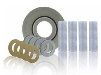
The PGE was designed to give operators an alternative to the failure prone phenolic-based isolating gaskets. Based on its construction, the PGE will provide a superior, long-lasting solution when compared to phenolic-based designs. The PGE is available in both full-face (Type E) and ring style (Type F) configurations. Depending upon the sealing element selected, the PGE is rated for most all hydrocarbon and water service applications.
