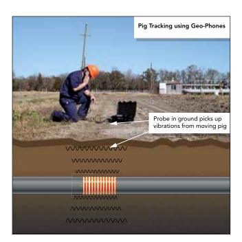
Geophones greatly amplify the vibrations of the pig rubbing against the wall of the pipe allowing the user to hear the pig coming from sometimes miles away.
