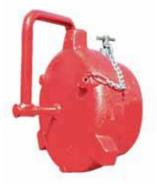
Our Figure 500 closure design combines simplicity and reliability through the use of a rugged, modified ACME thread to fasten the cap to the hub. The pressure seal is achieved by an O-ring set in the face of the hub. Figure 500 closures are manufactured in sizes 2'- 14."
