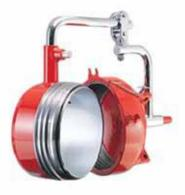
Our Figure 500R closure was designed for larger diameter closure applications and is machined with a bevel seat. The bevel seat on the hub provides the operator an accurate stabbing section and reduces the risk for the thread and seal damage. All of our Figure 500R closures also have a minimum of 3" thread lengths for greater safety and mechanical sealing integrity. Our Figure 500R design is available in sizes 16"-54," with closure horizontal hinges swing left or right for sizes 16" and above.
