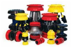
Steel-Body pigs, or Mandrel pigs, are heavy duty pigs which can be configured in a number of ways to provide maximum cleaning, sealing and sweeping power. These pigs can travel long distances and the urethane cups and discs are replaceable which makes them an economical option for many pipeline operators.
