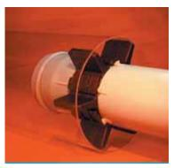
The Ranger II<sup>®</sup> is a completely non-metallic casing isolator/ spacer system that uses molded segments to encircle the carrier pipe. Each segment includes at least one molded-in runner and one slide lock. Customers may choose from any one of five different size bands to allow correct sizing for carrier pipe O.D. ranges from 0.83" up to 37.60" in diameter.
